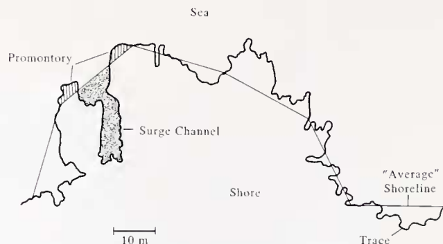
Figure 3. An example showing the traced shoreline (thick line), "average" shoreline at a particular scale (thin line segments), and the surge channel and promontory portions for a single segment of the average shore. This shoreline was traced from an aerial photograph of the shore at Hopkins Marine Station.
